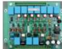
'All in One PLC card' for Mechanical Loom
