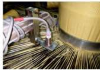
"Weft Break Detection" for avoiding Fabric Wastage
