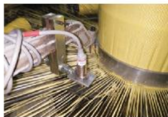
"Weft Break Detection" for avoiding Fabric Wastage
