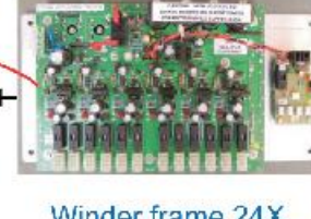
Winder frame 24X Power Supply card 'Synchronizer' Auto & Manual Avoids Total Frame Failure
