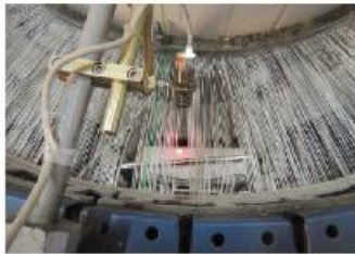
"Weft End Detection" for reducing tape wastage
