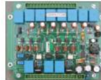
"Weft Break Detection" for avoiding Fabric Wastage
