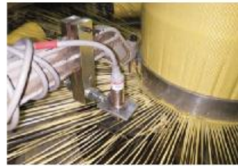
"Weft Break Detection" for avoiding Fabric Wastage
