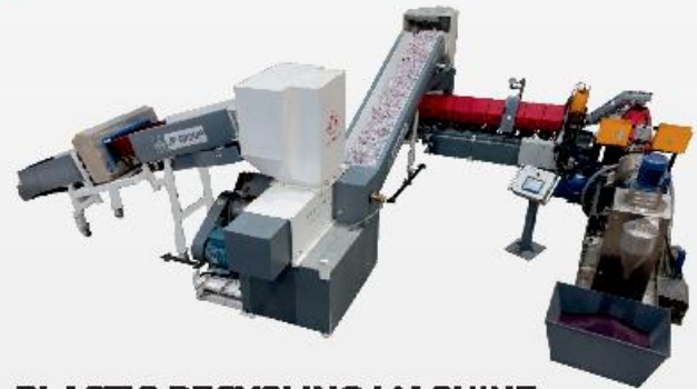
PLASTIC RECYCLING MACHINE Output Range: 100-450 Kg/Hr Suitable for: PP, BOPP, HDPE, LDPE & HIPS
