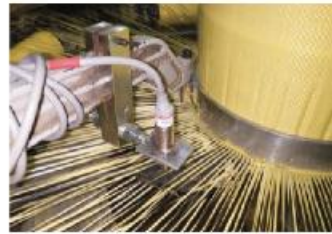
"Weft Break Detection" for avoiding Fabric Wastage
