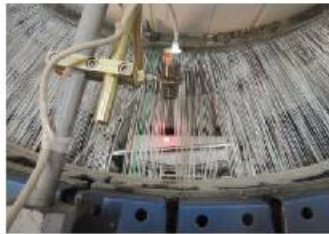
"Weft End Detection" for reducing tape wastage
