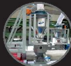
GSM control for Extrusion Lamination
