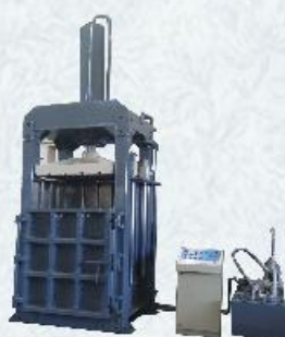
Hydraulic Bale Press For FIBC (Jumbo Bag)
