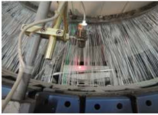
"Weft End Detection" for reducing tape wastage
