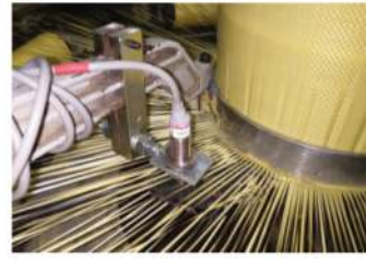
"Weft Break Detection" for avoiding Fabric Wastage
